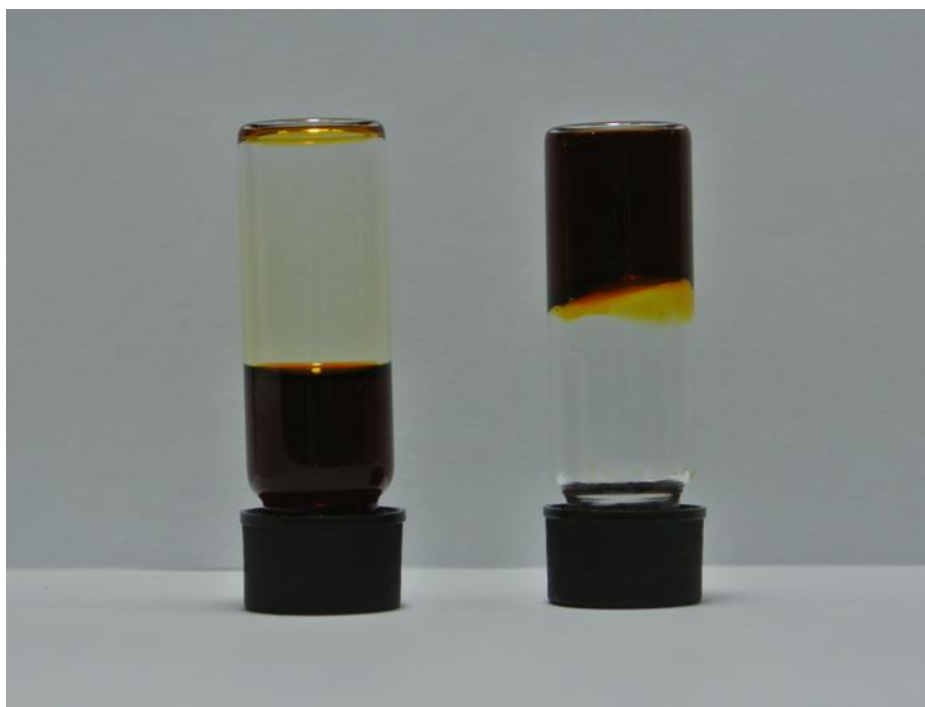
Figure S12. Photograph of liquid (left) and gel (right) electrolytes used in the PC part.
